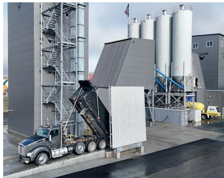
Getting ready for the first batch! The Osprey and the Falcon (Simem Wetbeton 180S plants). Aggregate loading areas incorporate hydraulically operated lids to protect materials from weather.
