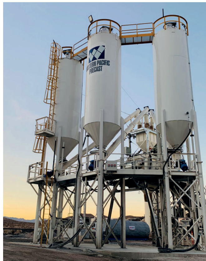
Eagle 7000 plant with a capacity up to 235 cu.yd./hr., fully equipped with a 6 cu.yd. compacted concrete output twin shaft mixer. Another beautiful morning for production.
